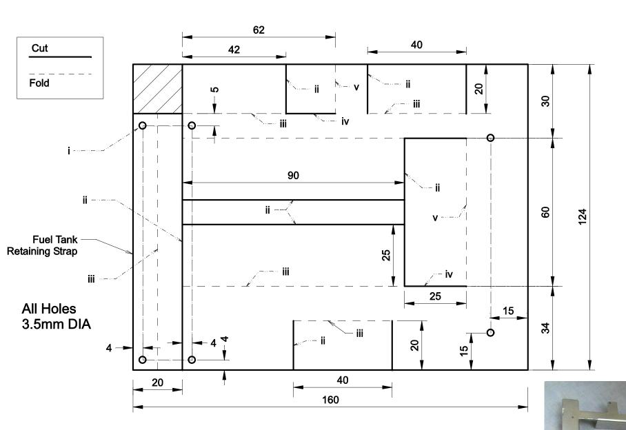
Cut/Fold Order i Drill Holes ii Cut iii Fold iv Cut v Fold
