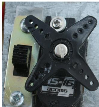
**Speed Controller:** You don't really need one, as you will be going flat out all the time. The supplied slide switch can be operated by the servo to give forward and reverse, as pictured. We do stock a limited number of digital speed controllers available at cost.
